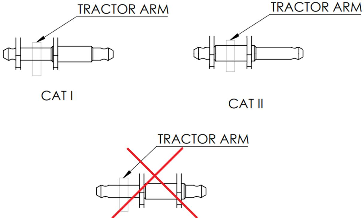
1. Fasten the tractor drawbars to the skidding winch.
